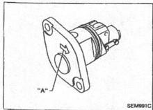
18. Install camshaft position sensor.
